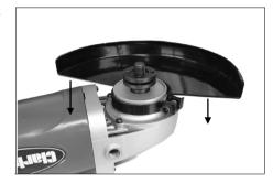
Rotate the disc guard to the required position and secure by tightening the screw.
